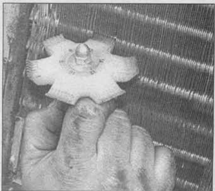
15.8 Straighten and clean bent condenser fins with a fin comb (available at most auto parts stores)
