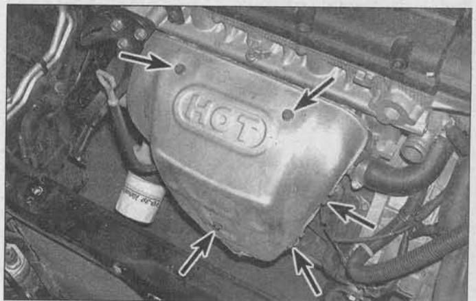
9.2a To detach the exhaust manifold heat shield from the exhaust manifold on 1996 through 2000 models, remove these seven bolts (arrows) (two bolts, on right side of shield, not visible in this photo)
