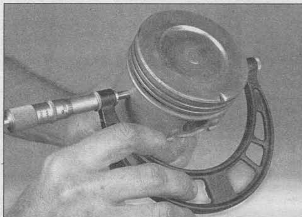
18.11 Measure the piston diameter at a 90-degree angle to the piston pin and at the specified distance from the bottom of the piston skirt
