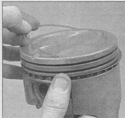
23.9b DO NOT use a piston ring installation tool when installing the oil ring side rails
