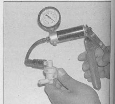
18.15 To test the two-way valve, hook up a hand-held vacuum pump and verify that air can travel through the valve in the direction of the arrow, but not in the opposite direction
