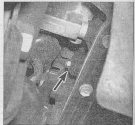
5.1 The knock sensor (arrow) is located on the front of the block; to detach the sensor from the block, remove the sensor retaining bolt
