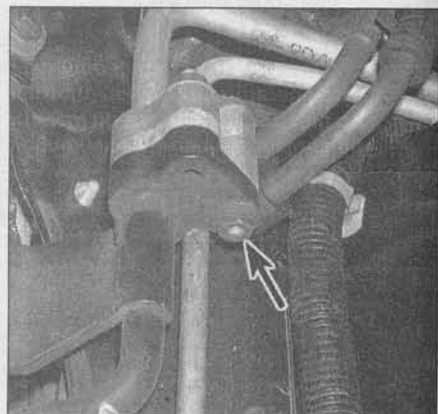
13.4b To disconnect the other line from the condenser, remove this nut (arrow)
