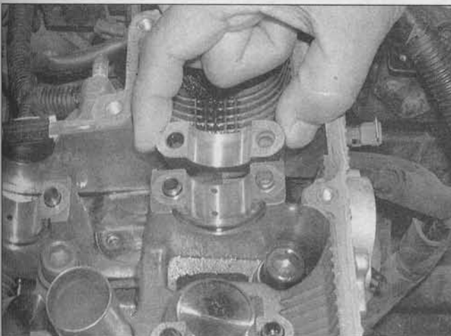
21.1 Inspect the camshaft bearing surfaces in the cylinder head for pits, score marks and abnormal wear - if damage is noted, the cylinder head must be replaced
