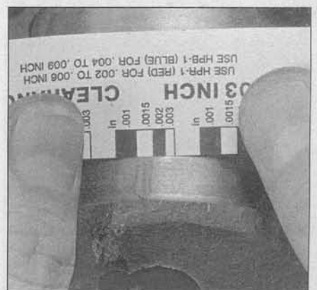
24.15 Measuring the width of the crushed Plastigage to determine the main bearing oil clearance (be sure to use the correct scale - standard and metric ones are included)
