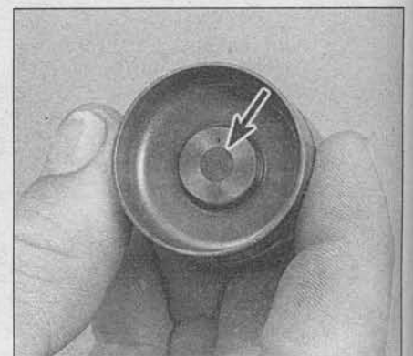
21.6b Also check the valve stem contact area of the lifter
