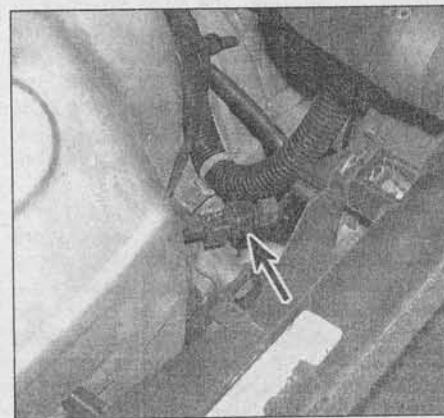
12.2a Crankshaft Position (CKP) sensor electrical connector (arrow)
