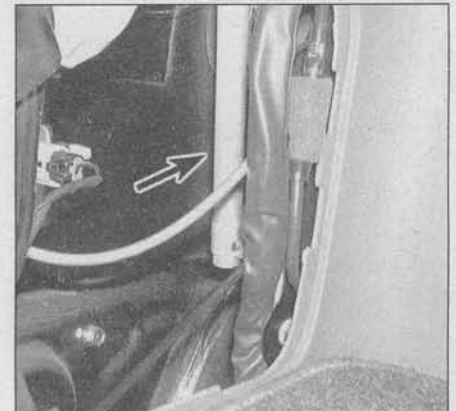
12.4 The antenna base is accessible with the trim panel removed
