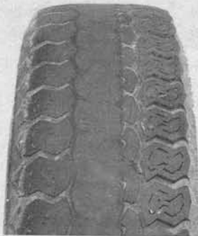
INCORRECT TOE-IN OR EXTREME CAMBER
