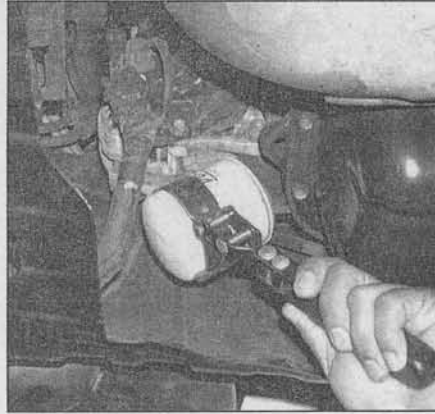
8.12 The oil filter is usually on very tight and will require a special wrench for removal - DO NOT use the wrench to tighten the new filter
