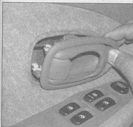
15.3c . . . rotate the handle assembly out of the trim panel, then disconnect the linkage rod
