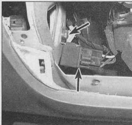
16.1 The Multipoint Fuel Injection (MFI) control relay is located under the steering column (trim panel and reinforcement removed); to remove the MFI control relay, unplug the electrical connector and remove this retaining bolt (arrow)
