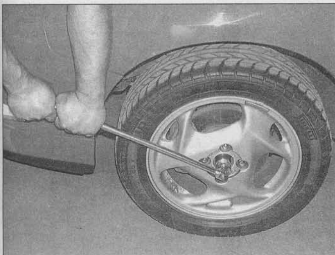
11.2 Loosen the driveaxle/hub nut with a long breaker bar - depending on the design of the wheel, it may be necessary to install the spare wheel and tire to access the hub nut
