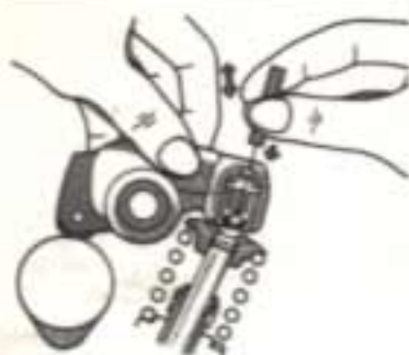
10.1 When performing the freeplay test, make sure the adjuster that's being tested has the corresponding camshaft lobe pointing away from the rocker arm (closed valve).
