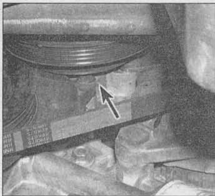
8.4 The water pump weep hole (arrow) is located on the underside of the pump
