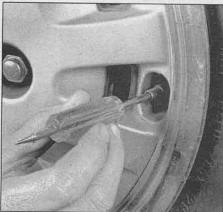
5.4a If a tire loses air on a steady basis, check the valve core first to make sure it's snug (special inexpensive wrenches are commonly available at auto parts stores)
