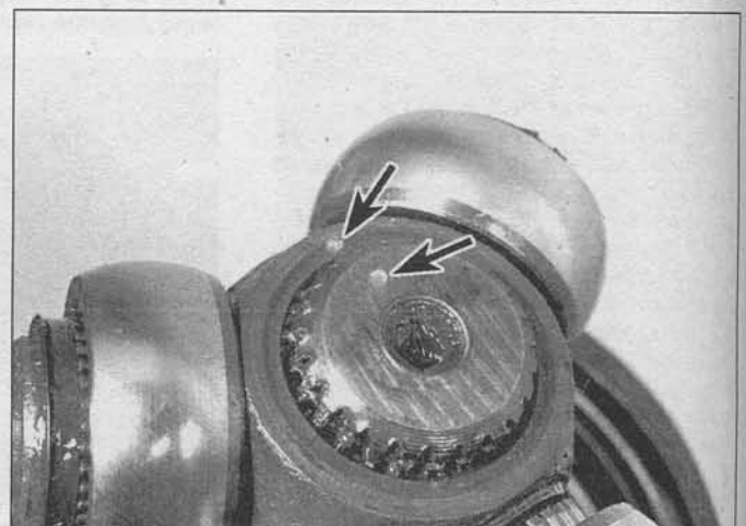
12.5 Use a center punch to place marks (arrows) on the tri-pot and the driveaxle to ensure that they are properly reassembled
