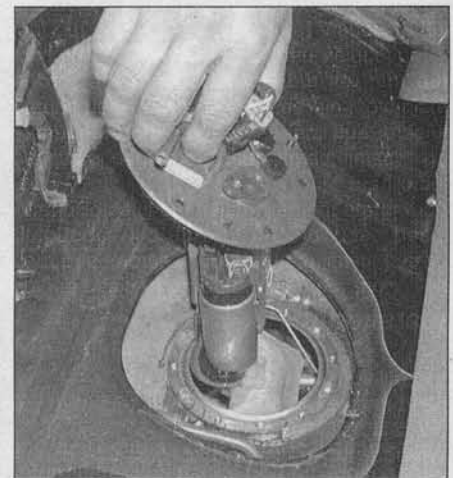
5.6 Remove the fuel pump/fuel sending unit assembly from the fuel tank
