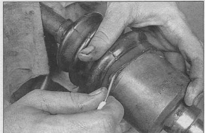
12.14 Equalize the pressure inside the boot by inserting a small, dull screwdriver between the boot and the housing
