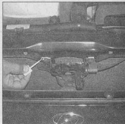
10.9 Before adjusting the hood latch horizontally or vertically, mark its position, then loosen the bolts
