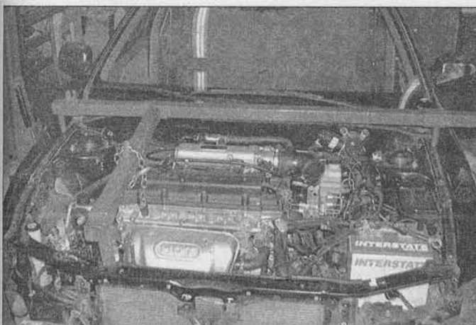
6.8 Install an engine support brace across the engine compartment
