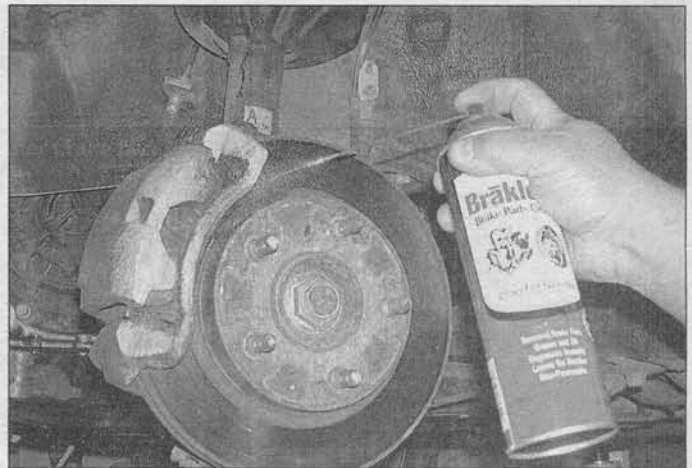
3.6a Before removing anything, spray the disc, caliper and brake pads with brake system cleaner to remove the dust produced by brake pad wear - DO NOT blow the dust off with compressed air!
