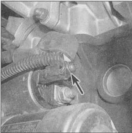
4.4a To disconnect the positive battery cable from the starter solenoid terminal, remove this nut (arrow)
