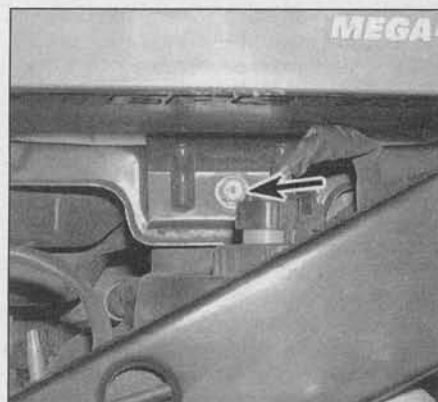
3.4 To remove the battery from the battery tray, remove the battery hold-down clamp bolt (arrow) and clamp, and then lift out the battery
