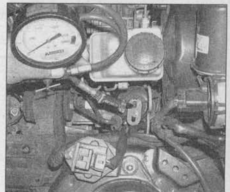
3.12b ... and then use it to connect a fuel pressure gauge to the fuel filter
