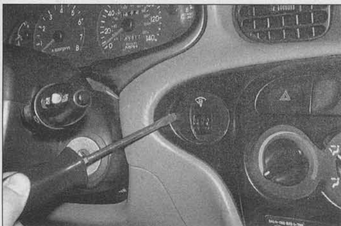
9.2a Pry the dashboard light control unit out of the center instrument panel bezel (2000 and earlier model shown)
