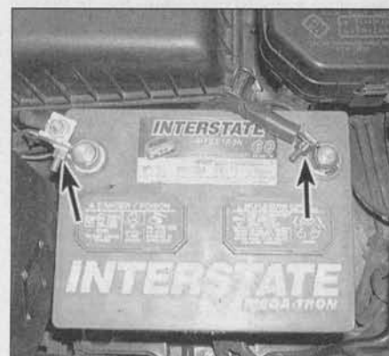
3.2 Loosen the negative cable clamp nut (right arrow) and remove the negative battery cable from the negative battery post. Isolate the cable end to prevent it from accidentally coming into contact with the battery post. Loosen the positive cable clamp nut (left arrow) and remove the positive battery cable from the positive battery post
