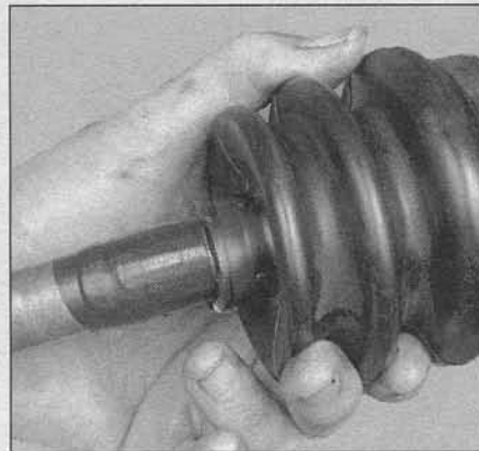
12.10 Wrap the splined area of the axle shaft with tape to prevent damage to the boot(s) when installing it
