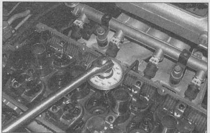
10.23b Use an angle-measuring gauge to angle-torque the cylinder head bolts
