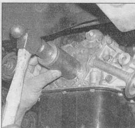
5.6 Tap the new seal into place with a large socket or piece of pipe and a hammer - the outside diameter of the pipe or socket should be slightly smaller than the seal
