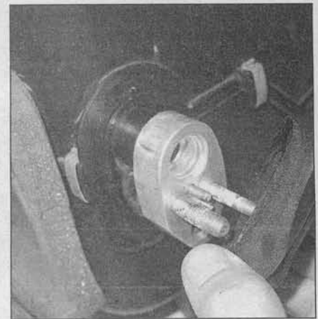
16.9 Remove the sponge pad which insulates the evaporator inlet and outlet pipes
