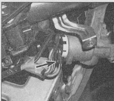
8.3 The ignition switch is retained in the lock cylinder housing by one screw
