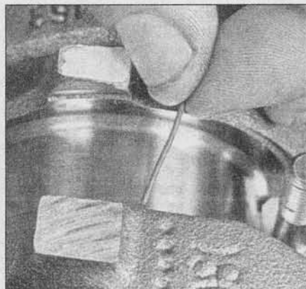
26.13 Lay the Plastigage strips on each rod bearing journal, parallel to the crankshaft centerline
