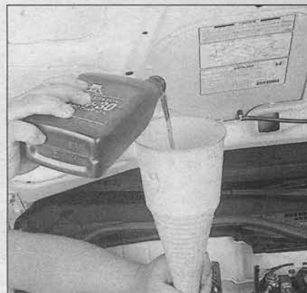
17.2b . . . so you can easily add lubricant to the transaxle from above
