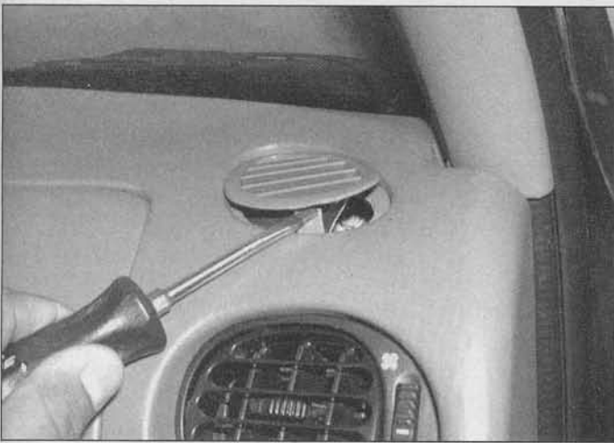
30.8c Pry off the grilles at the top corners of the instrument panel for access to . . .
