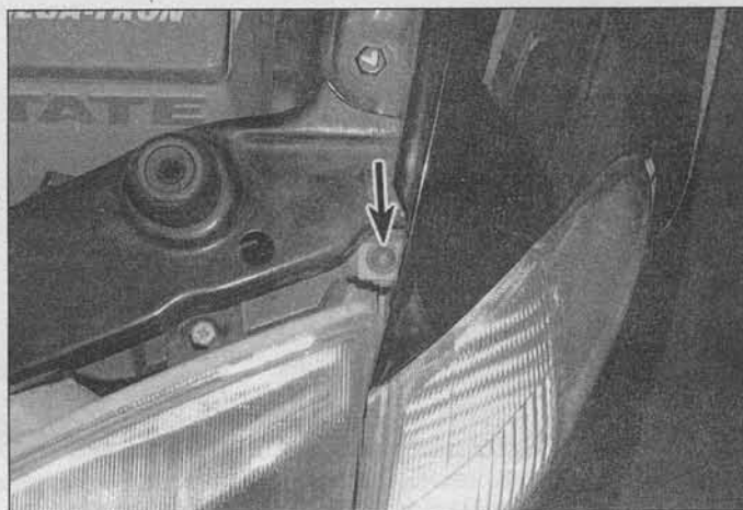
16.2a After removing the retaining screw . . .
