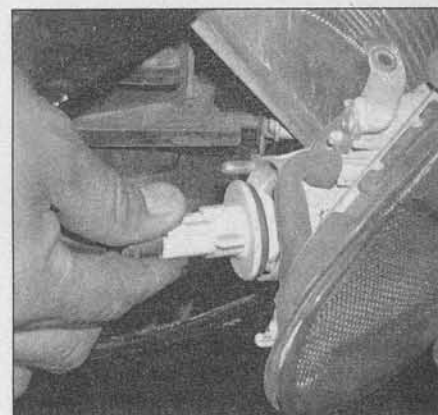
16.2b . . . pull the turn signal/park light housing straight out of the body
