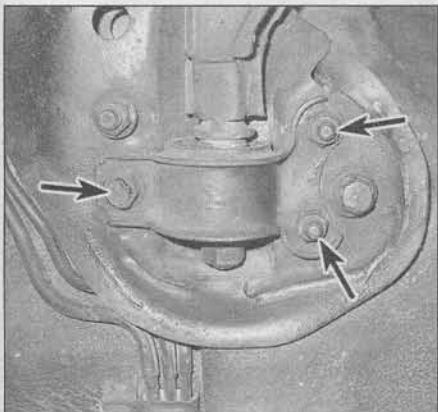
7.6 Remove the rear pivot bushing bolt and nuts (arrows) (2000 and earlier models shown)
