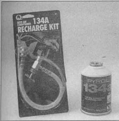
12.11 R-134a refrigerant and recharge kits are available from auto parts stores; follow the instructions that come with the kit
