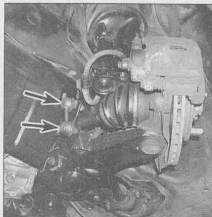
24.9c Check the stabilizer bar links (arrows) for looseness at the front and rear of the vehicle; also check the stabilizer bar bushings
