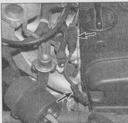
11.1 The Camshaft Position (CMP) sensor (lower arrow) is located at the right rear corner of the cylinder head; the electrical connector (upper arrow) is located right above the injector for cylinder No. 1
