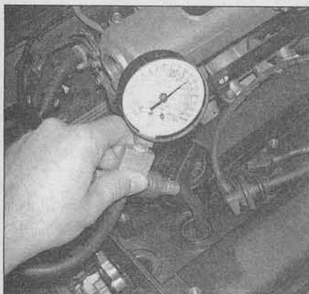
3.5 Use a compression gauge in the number one spark plug hole to assist in finding TDC
