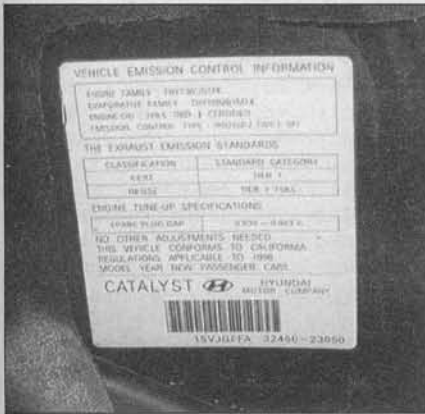
1.7a The Vehicle Emission Control Information (VECI) label is located in the engine compartment and contains information on the emission devices on your vehicle
