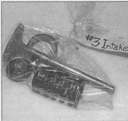
9.2 A small plastic bag, with an appropriate label, can be used to store the valve train components so they can be kept together and reinstalled in the original positions
