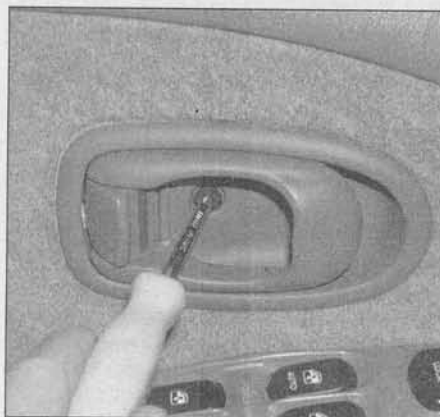
15.3a Remove the inner door handle screw
