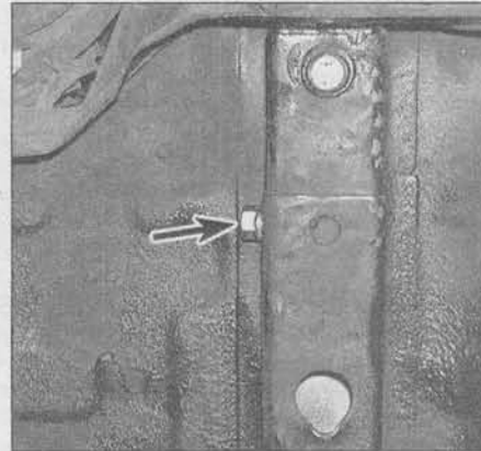
12.10b The remaining bumper bolts on station wagon models are located under the rear compartment on each side (arrow)
