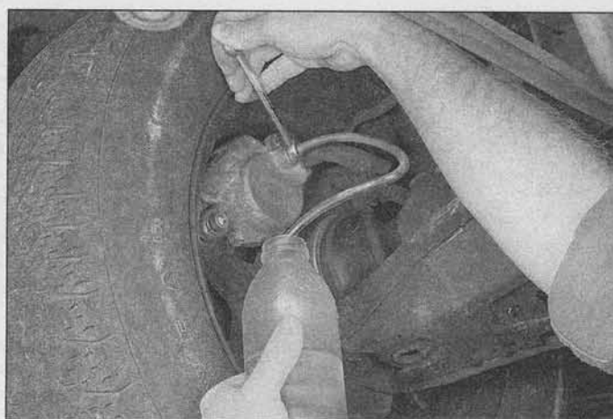
10.8 When bleeding the brakes, a hose is connected to the bleed screw at the caliper or wheel cylinder and then submerged in brake fluid - air will be seen as bubbles in the tube and container (all air must be expelled before moving to the next wheel)
