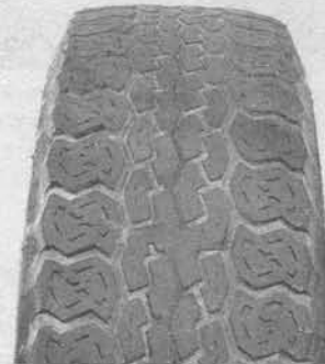
FEATHERING DUE TO MISALIGNMENT
