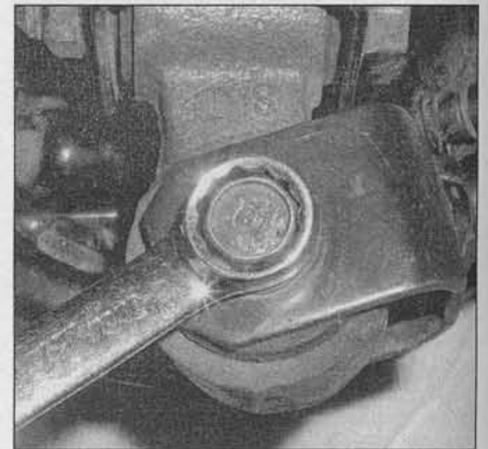
13.4 Remove the bolt that attaches the rear end of the trailing arm to the knuckle
