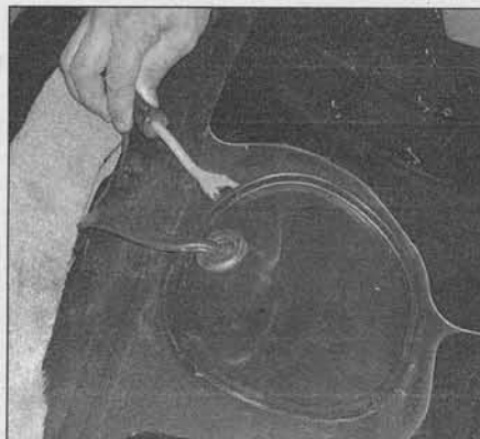
2.2 To remove the fuel pump access cover, break loose the sealant with a suitable prying tool
