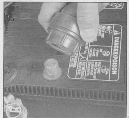
11.8b Regardless of the type of tool used on the battery posts, a clean, shiny surface should be the result (the inside of the clamp is tapered to match the taper on the post, so don't remove too much material)
