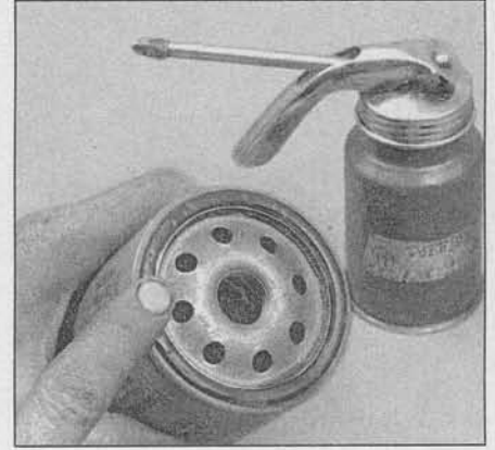
8.14 Lubricate the oil filter gasket with clean engine oil before installing the filter on the engine
