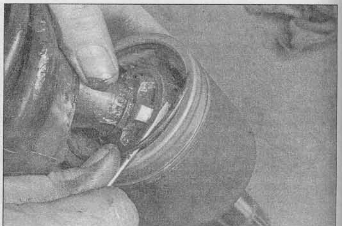
12.18 Pry the wire retainer ring from the CV joint housing with a small screwdriver
