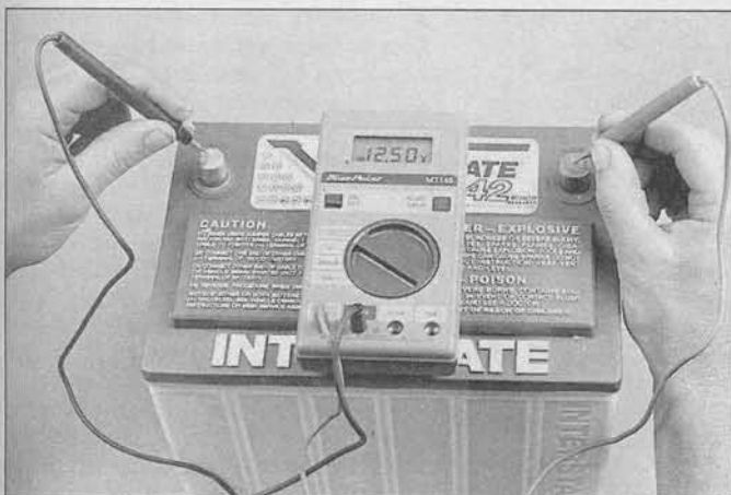
3.1b To test the open circuit, or standing, voltage of the battery, connect the black probe of the voltmeter to the negative terminal and the red probe to the positive terminal of the battery. A fully charged battery should indicate about 12.5 volts, depending on the ambient air temperature
