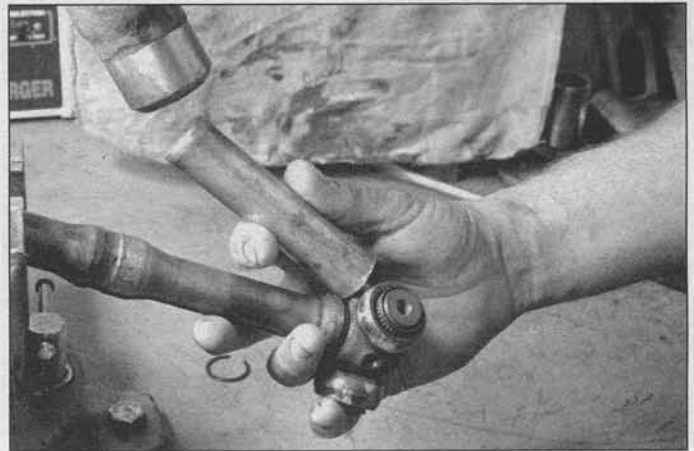
12.7 Drive the tri-pot joint from the axle shaft with a brass punch and hammer – make sure you don't damage the bearing surfaces or the splines on the shaft
