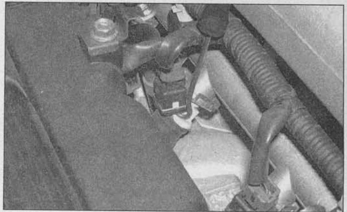
15.4 To disconnect the fuel injector electrical connectors, release the lock wire on each connector by pulling it out to its "released" position (it will snap out and remain out until depressed) and then unplug the connector
