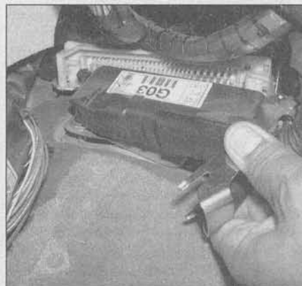
3.5 . . . pull down the PCM, then disconnect the electrical connector and remove the PCM
