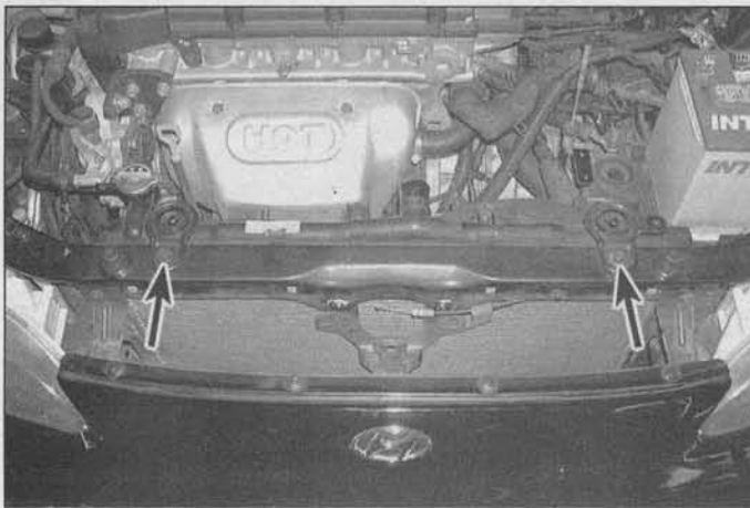
4.8 To detach the radiator from the crossmember, remove these mounting bolts (arrows)
