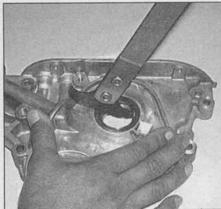
12.10 Remove the old crankshaft front seal from the oil pump housing with a seal removal tool
