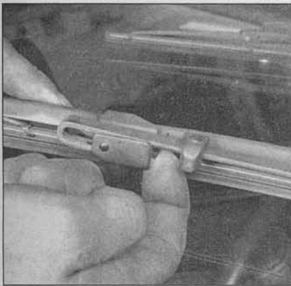
10.6 Press in on the tab and push the blade assembly out of the hook at the end to remove it
