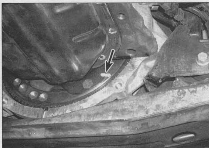
6.15a Mark the torque converter-to-drive plate relationship (arrow) ...
