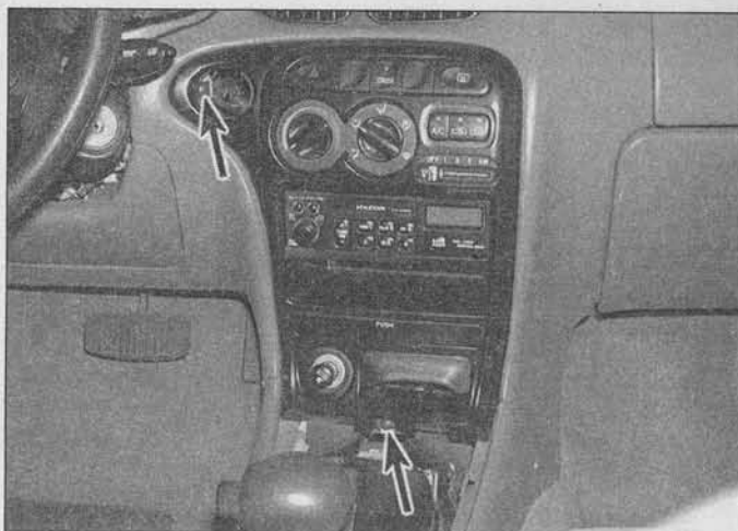
28.11a Remove the screws in the dashboard light control opening and at the base of the bezel (arrows) (2000 and earlier models)
