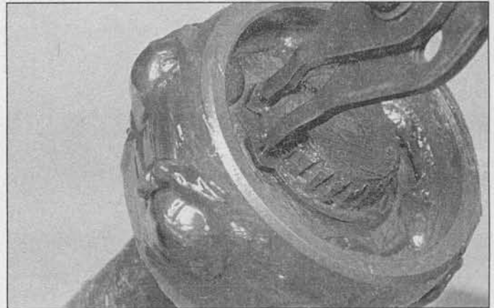
12.20 Remove the snap-ring from the end of the axle shaft
