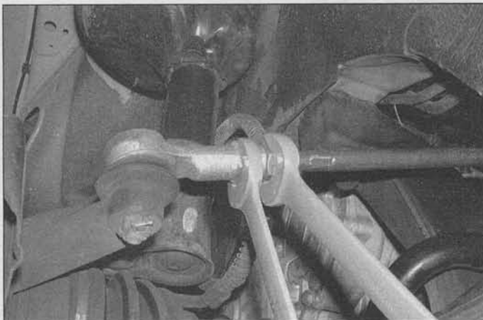
16.2 Loosen the jam nut, then mark the position of the tie-rod end in relation to the threads
