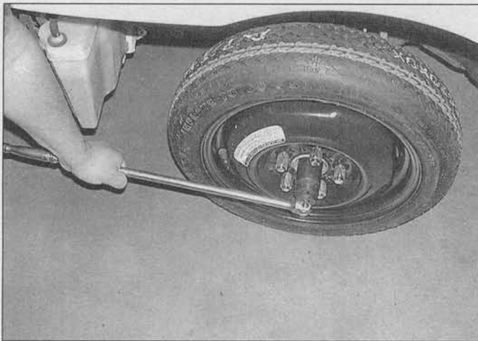
4.2 Use a breaker bar and socket to loosen the driveaxle/hub nut - install the spare tire onto the hub if the nut is not accessible through the wheel
