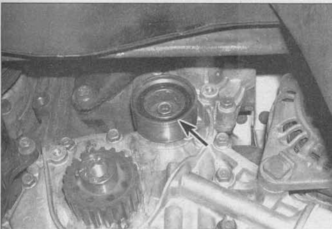
5.11 Remove the timing belt idler pulley bolt (arrow) and then remove the idler pulley
