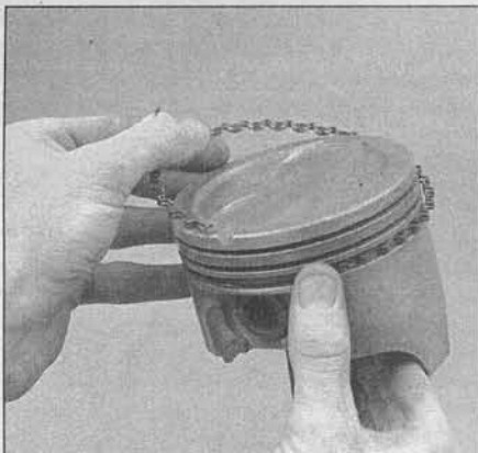
23.9a Installing the spacer/expander in the oil control ring groove
