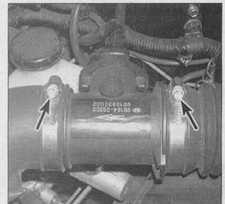
4.1 The MAF sensor is located in the intake duct between the air cleaner housing and the throttle body; to remove it, simply loosen the hose clamp screws (arrows)
