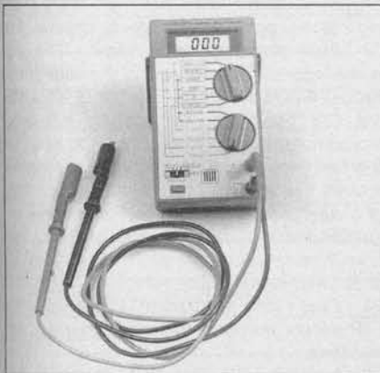
2.1 Digital multimeters can be used for testing all types of circuits; because of their high impedance, they are much more accurate than analog meters for measuring low-voltage computer circuits
