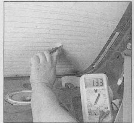
20.8 To find the break, place the voltmeter negative lead against the defogger ground terminal, place the voltmeter positive lead with the foil strip against the heat wire at the positive terminal end and slide it toward the negative terminal end - the point at which the voltmeter deflects from several volts to zero volts is the point at which the wire is broken
