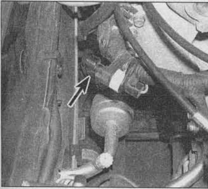
3.3a The fuel pump check connector (arrow) is located at the rear of the engine compartment, behind and below the air intake plenum
