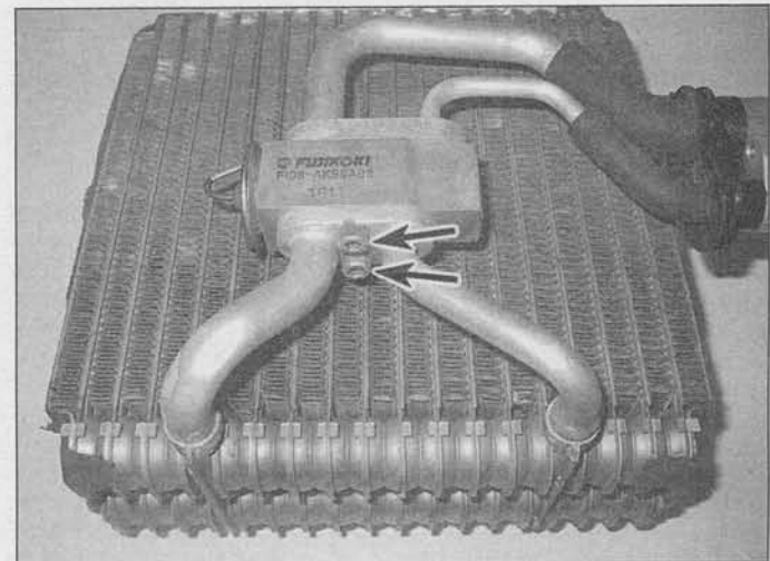
16.12 After removing the evaporator from the lower case, remove the expansion valve retaining bolts (arrows) and then separate the expansion valve assembly from the evaporator
