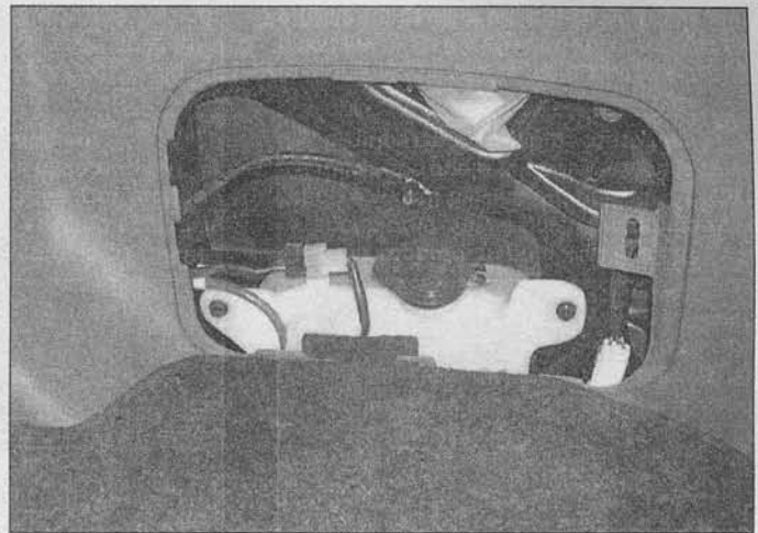
4.14b Flip up the cap to add fluid to the rear window washer reservoir
