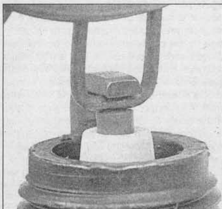
19.5a Spark plug manufacturers recommend using a wire-type gauge when checking the gap - if the wire does not slide between the electrodes with a slight drag, adjustment is required
