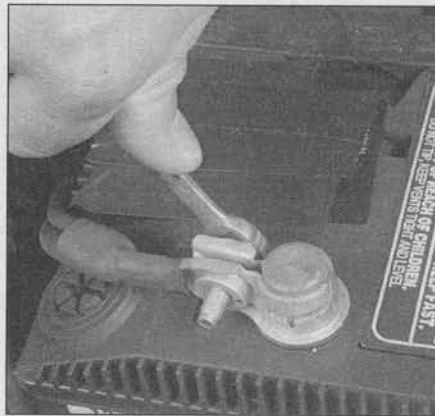
11.7b Removing the cable from a battery post with a wrench - sometimes special battery pliers are required for this procedure if corrosion has caused deterioration of the nut hex (always remove the ground cable first and hook it up last!)
