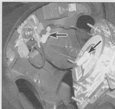
14.4 Carefully lift the airbag module and disconnect the airbag electrical connectors (arrows)
