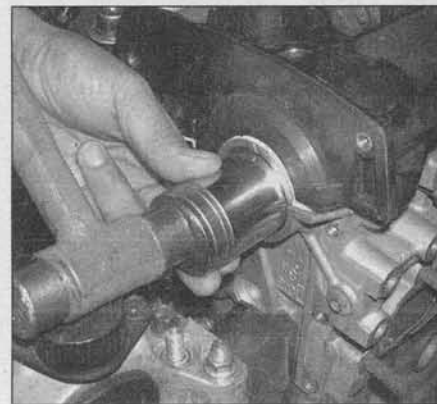
7.3 Using a socket with an outside diameter slightly smaller than the outside diameter of the seal, carefully drive the new seal into place with a hammer
