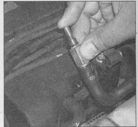
21.4 With the engine running at idle, remove the PCV valve and verify that vacuum can be felt at the end of the valve
