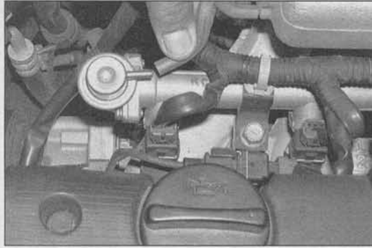
3.16 Disconnect the vacuum line from the fuel pressure regulator - the fuel pressure should immediately increase (2000 and earlier models only)
