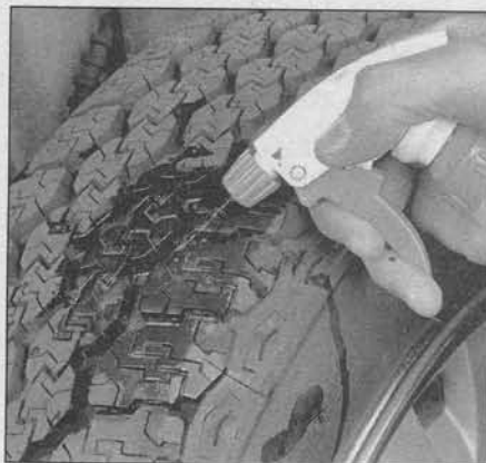
5.4b If the valve core is tight, raise the corner of the vehicle with the low tire and spray a soapy water solution onto the tread as the tire is turned slowly - leaks will cause small bubbles to appear
