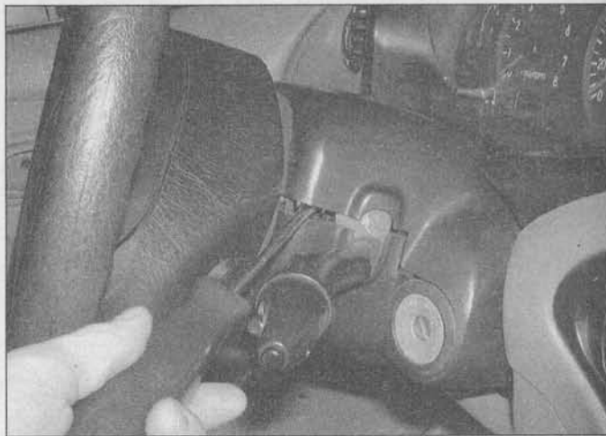
29.2 Remove the screws under the lower column cover, then use a screwdriver to detach and remove the upper and lower covers
