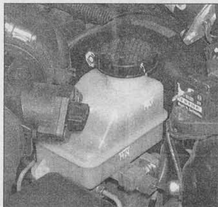
4.16 The brake fluid should be kept between the MIN and MAX marks on the reservoir - turn and lift up the cap to add fluid
