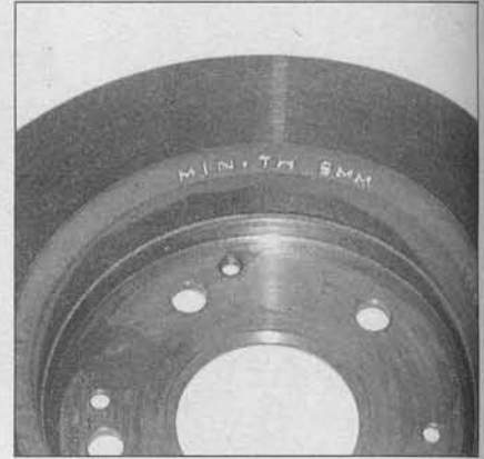
5.5a The minimum allowable thickness is stamped into the disc (typical)
