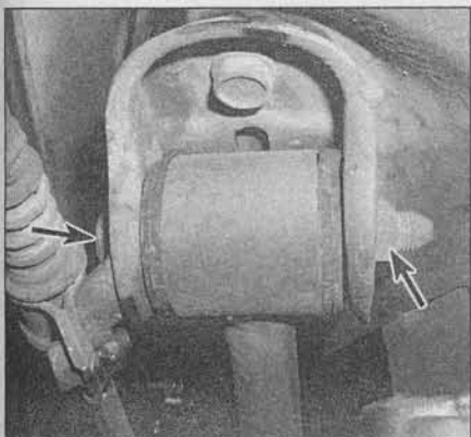
13.5 To disconnect the forward end of the trailing arm from the body, remove the nut and pivot bolt (arrows)
