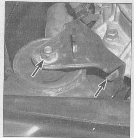
15.4c Front roller stopper nuts and bolts (arrows) (other bracket to transaxle bolt not visible in this photo)
