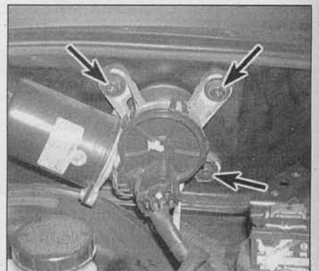
17.4 Unscrew the bolts (arrows) and remove the wiper motor
