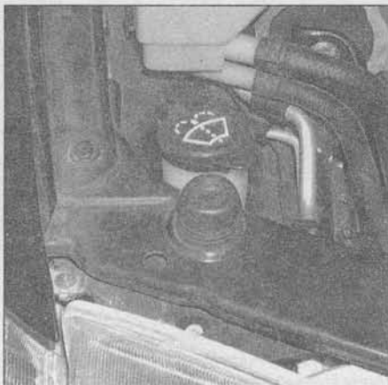
10.10 To adjust the vertical height of the front edge of the hood so that it's flush with the fenders, turn each hood bumper clockwise (to lower the hood) or counterclockwise (to raise the hood)
