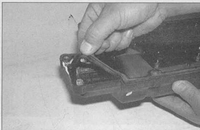
4.7 Remove the valve cover gasket from the valve cover
