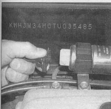
15.2a To unplug the ISC electrical connector, depress the wire retainer and pull off the connector (1996 through 2000 model shown, 2001 models similar)
