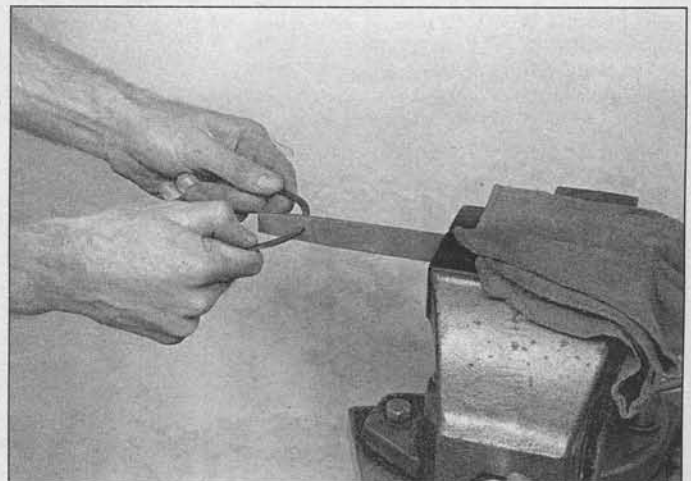
23.5 If the end gap is too small, clamp a file in a vise and file the ring ends (from the outside in only) to enlarge the gap slightly
