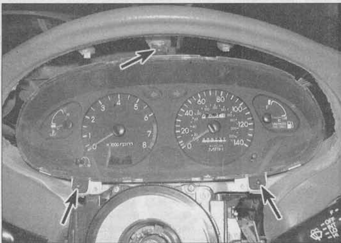
10.3a Remove the instrument cluster screws (arrows) then . . .
