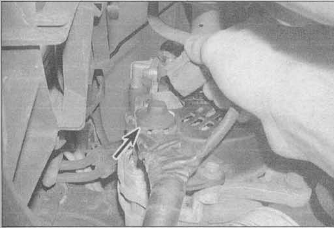
10.3 Unplug the big electrical connector from the alternator, remove the rubber plug (arrow) from the B+ terminal and then disconnect the wire from the B+ terminal
