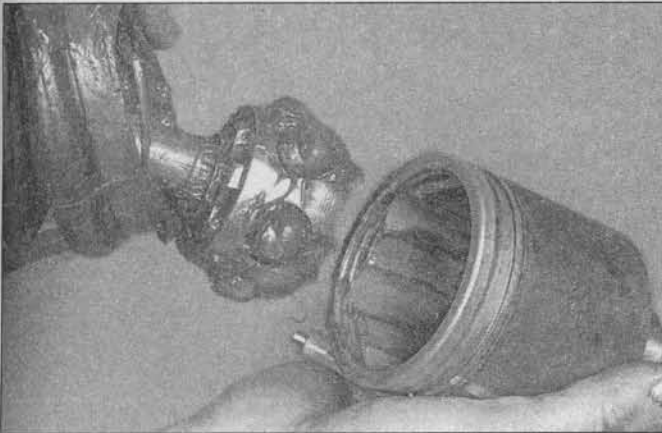
12.19 With the retainer removed, the CV joint housing can be pulled off the ball-and-cage bearing assembly
