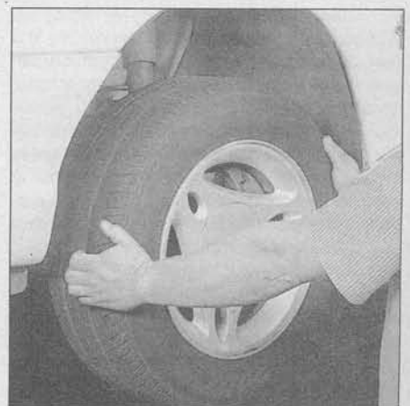
24.11 With the steering wheel in the lock position and the vehicle raised, grasp the front tire as shown and try to move it back-and-forth - if any play is noted, check the steering gear mounts and tie-rod ends for looseness
