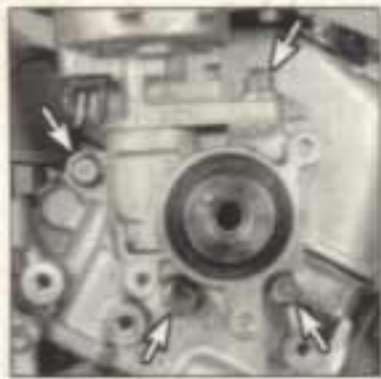
8.5a To remove the distributor drive adapter, remove the distributor hold-down nut (upper arrow), remove the distributor and remove the three adapter retaining bolts (arrows).
